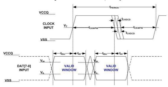
Figure 7.7 HS400 Device Data Input Timing
