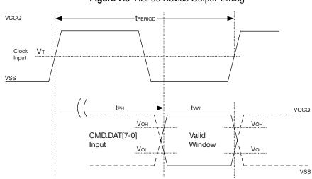
Figure 7.5 HS200 Device Output Timing
