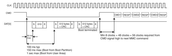
Figure 5.1 MultiMediaCard State Diagram (Boot Mode)
