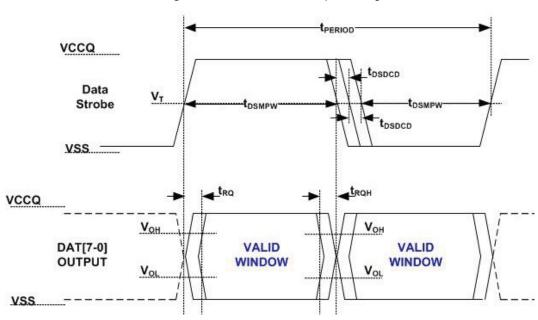
Figure 7.8 HS400 Device Output Timing
