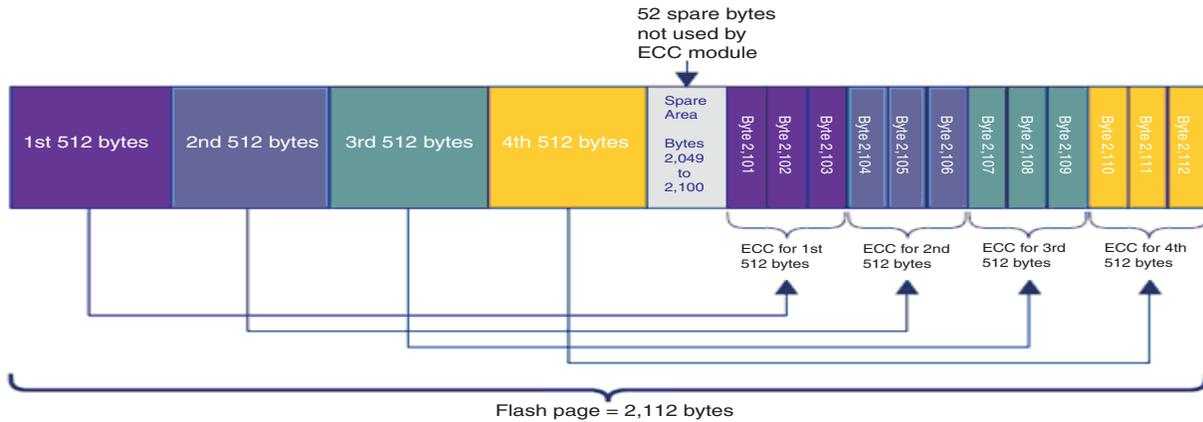
In this configuration the Hamming code requires 3 bytes of ECC information for each 512-bytes sector, or 12 bytes (96 bits) of ECC encoding information is required per 2 kB page.
